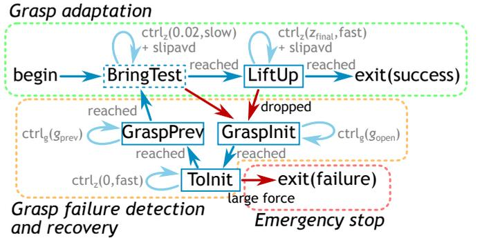
Fig. 3: Control scheme of the grasp adaptation. The detection of grasp failure and recovery, and emergency stop are unified.
