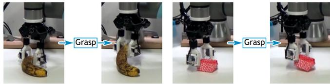
Fig. 4: Examples of uncertainty in poses of grasped objects that are caused by slippage during grasping.
