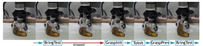
Fig. 9: Detection of drop and recovery to grasp the object again.
