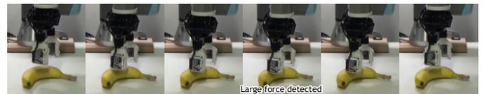
Fig. 10: Emergency stop in grasping a banana.
