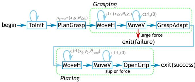
Fig. 6: Pick-and-place with the assistive utilities.
