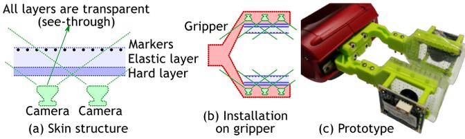
Fig. 1: Conceptual design of FingerVision (a, b) and its prototype installed on Baxter electric parallel gripper (c).
