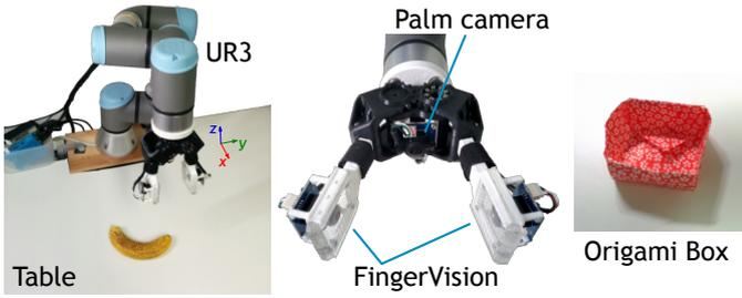
Fig. 5: Overview of the robot system.
